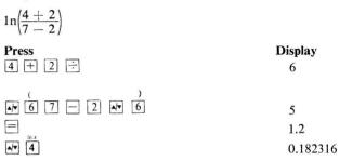
Do not attempt to enter a new number immediately after closing brackets (this should not in any case be necessary). Note: Pressing = does not close brackets
