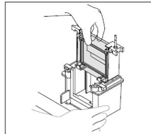
4. Press down the Electrode Assembly while closing the two cam levers of the Clamping Frame.
