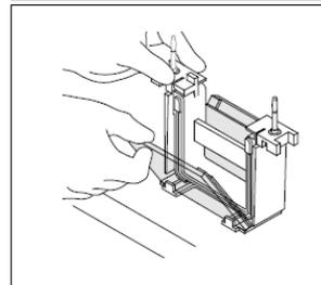
3. Slide Gel Cassette Sandwiches and Electrode Assembly into the clamping frame.
