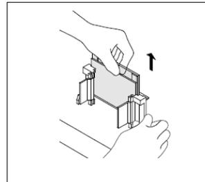
2. Place the Gel Cassette Sandwich into the Electrode Assembly with the Short Plate facing inward.
