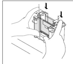
5. Lower the Inner Chamber into the Mini Tank.
