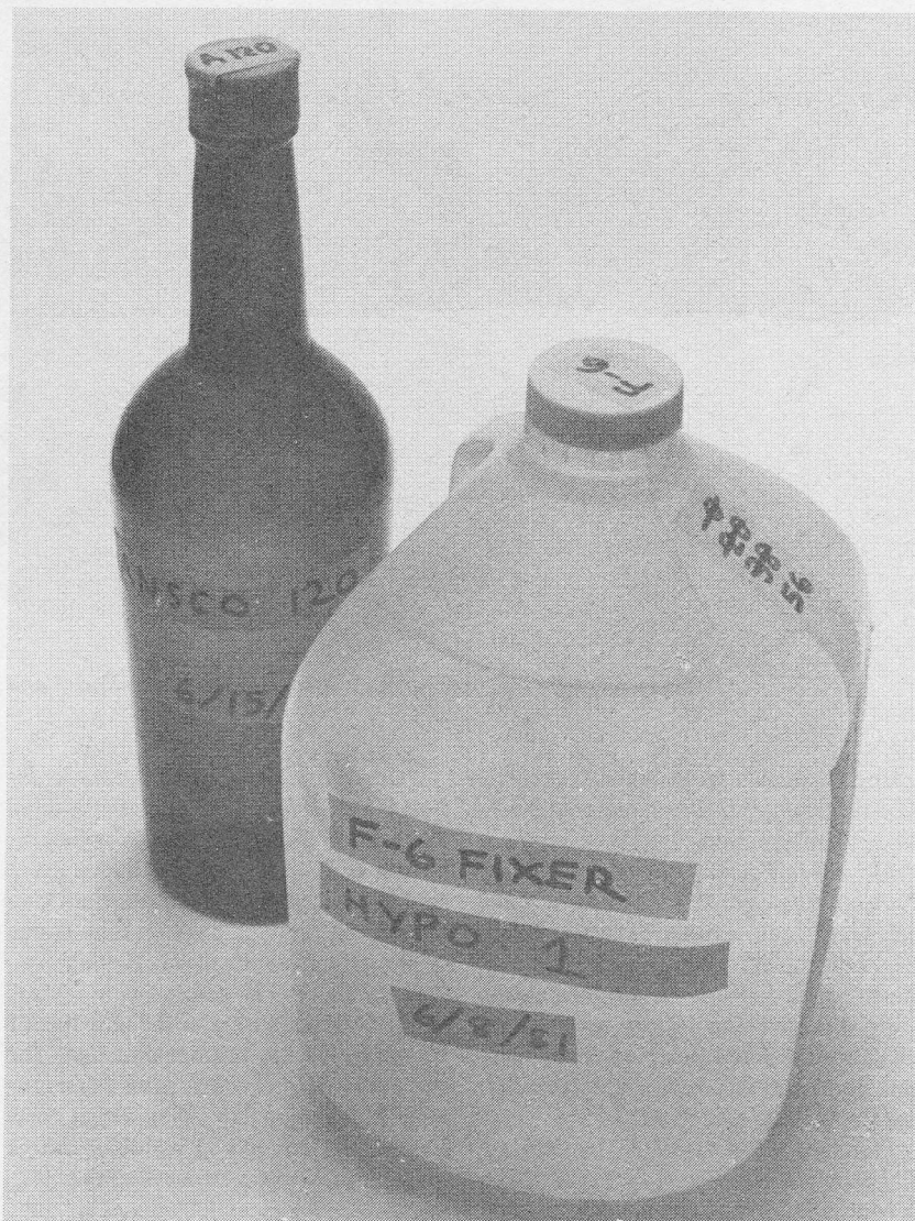
Author stores developer in glass bottles to reduce oxidation. For fixer this is not necessary. Note tally showing this fixer was used for 56 8x10-in. prints.
