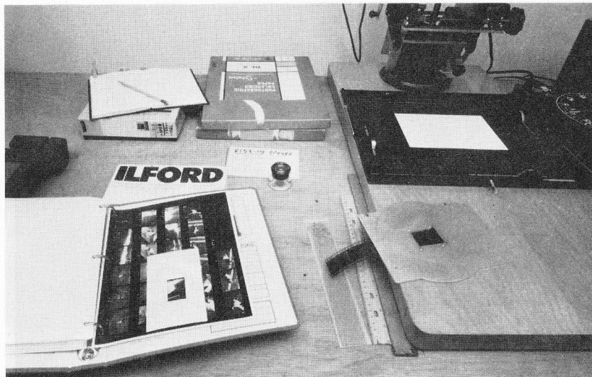
Enlarging table in use: a picture has been chosen from the contact proof sheet and the proper 35-mm negative has been placed in the carrier, emulsion-side down.
