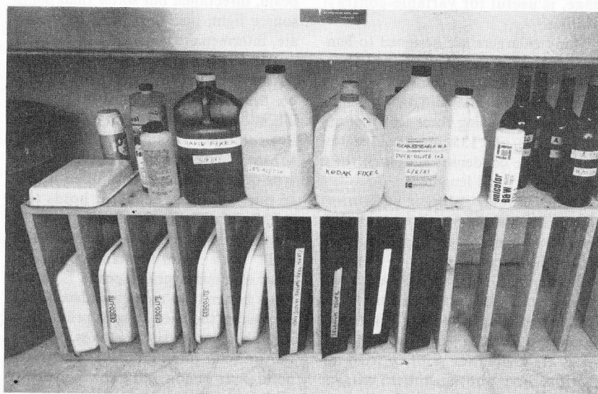
Tray rack and chemical shelf are on dry side under processing sink.
