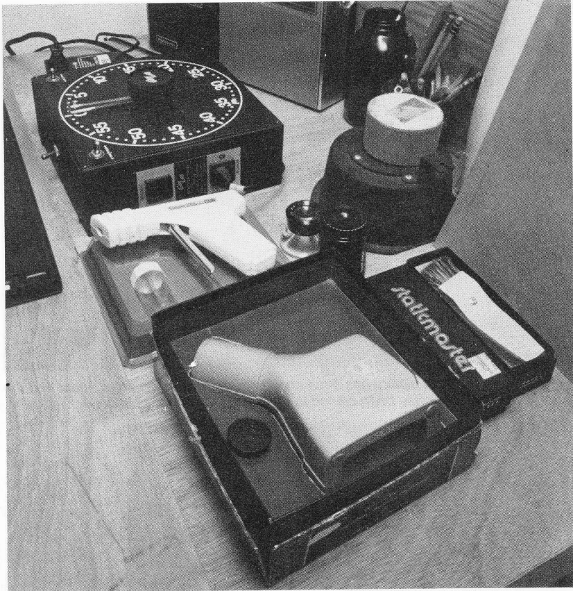
Next to enlarger are: timer, antistatic gun, brush, magnifiers, focusing magnifier, enlarging lens, cardboards, pencils, radio. Not visible is voltage stabilizer.
