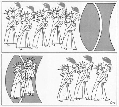
The two illustrations above show the effects of light loss in a lens due to its optical design as well as reflectance and absorption of the lens elements. Five lamp-bearing ladies may start on the quest for the film plane, but two become lost in the elements; the result is that only three ladies actually make it to their final destination. I would say that this lens has a transmittance of only 60 percent.
